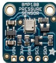
**Figure 5.** BMP 180 pressure sensor
