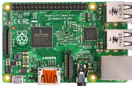
**Figure 4.** Raspberry Pi 2 (Model B)
