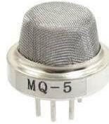
**Figure 7.** MQ5 Methane sensor
