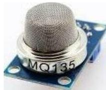
**Figure 9.** MQ135 Carbon dioxide sensor
